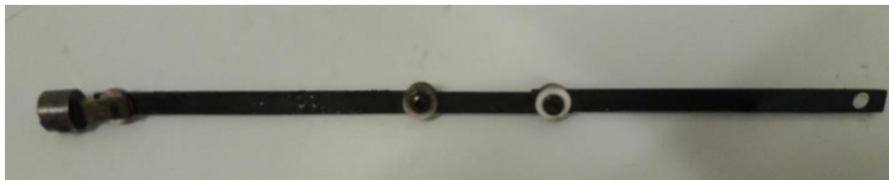
Figure 1: Illustration of three testing samples as used in each reactor for corrosion testing.
