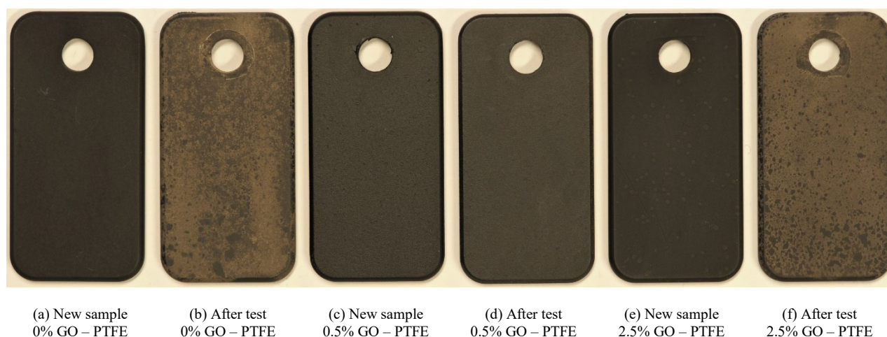
Figure 7: Photos of coupon samples with 0%, 0.5% and 2.5% GO – PTFE coatings un-tested (new) and after 250 °C corrosion tests in vapor phase.
