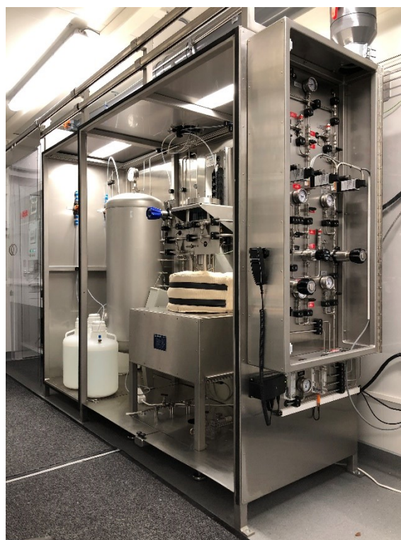
Figure 3: The autoclave experimental setup, including gas filling station (right) and H 2 S capture system (left).
