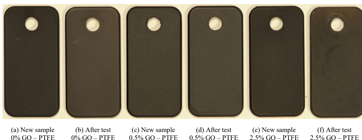
Figure 8: Photos of coupon samples with 0%, 0.5% and 2.5% GO – PTFE coatings un-tested (new) and after 250 °C corrosion tests in liquid phase.
