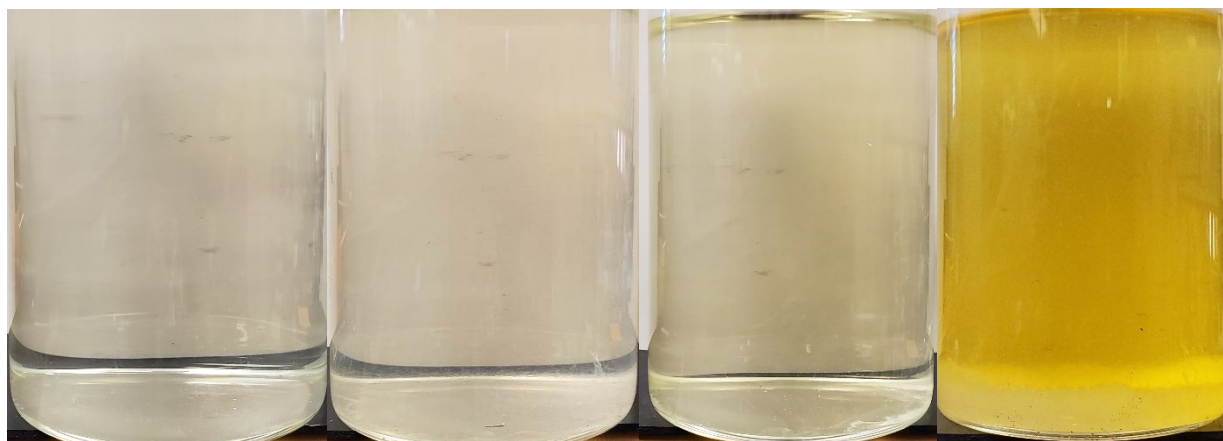
Figure 8: Images of 10 wt.% solutions of (left to right) inhibitor A prior to thermal treatment at 250 °C, inhibitor A after thermal treatment at 250 °C for one hour, inhibitor E prior to thermal treatment at 250 °C, and inhibitor E after thermal treatment at 250 °C for one hour. Note the formation of precipitant in inhibitor E after autoclaving.
