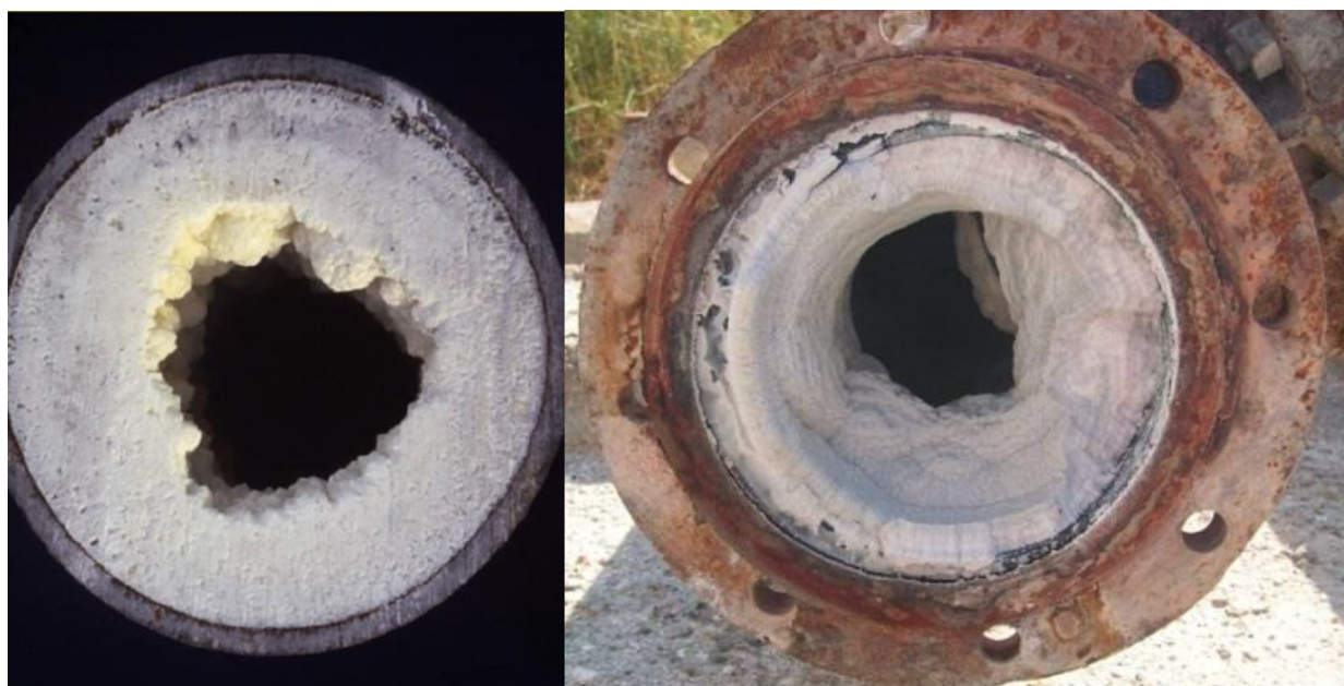
Figure 1: Examples of calcium carbonate deposition in a geothermal process. The image on the right is adapted from Haizlip et al., 2012.
