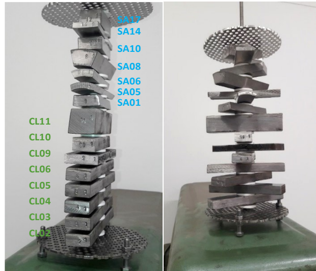
Figure 5: Assembled sample holders and position of samples listed in Table 3. The setup of both sample holders, for testing in 210°C and 450°C, were identical.
