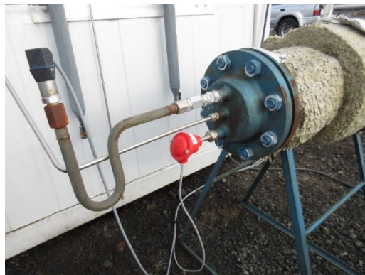
Figure 2: Outer experiment vessel, working at steam-pipe pressure and temperature.
