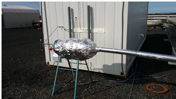
Figure 2: Outer experiment vessel, working at steam-pipe pressure and temperature.
