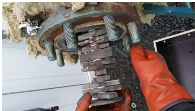
Figure 3: Insertion of samples in the outer vessel.
