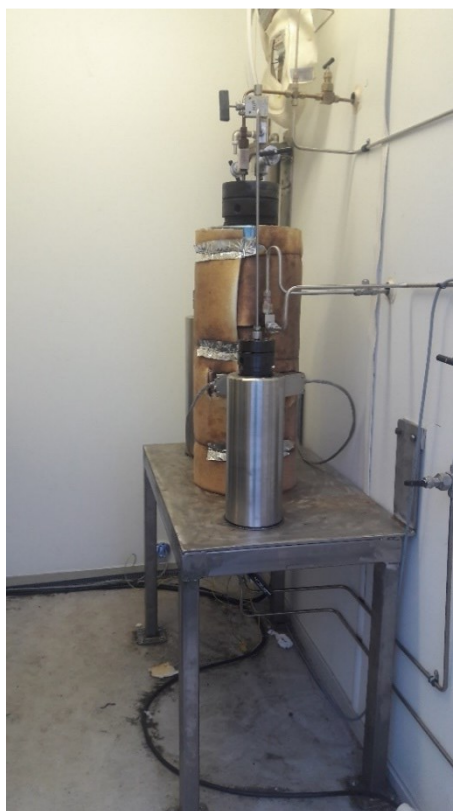
Figure 4: Side view of autoclave for testing at 450°C, support table and pipework. The needle valve near the wall, leading from the top of the autoclave, restricted the outflow of steam to maintain constant temperature and control effective heating.
