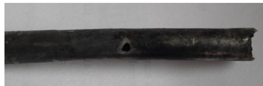
Figure 19: Extract of capillary tubing recovered after failure (CFE).
