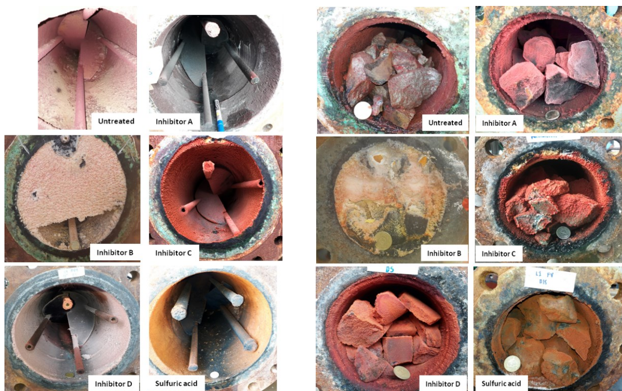
Figure 7. Resulting scale deposits on the retention vessels (left group) and formation vessels (right group) per test run
