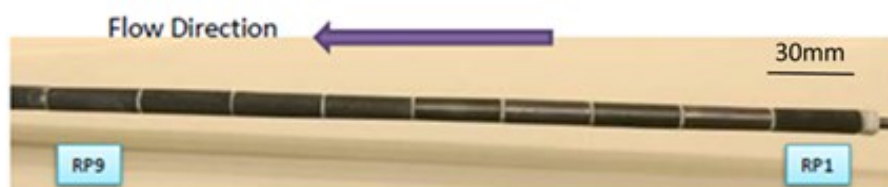
Figure 4: Cylinder coupon sample of the corrosion test loop system.
