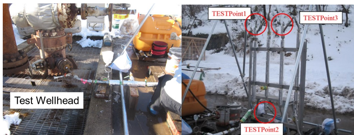
Figure 3: Corrosion test loop system at Yanaizu-Nishiyama geothermal field
