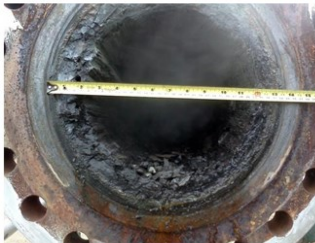
Figure 4: Well D Branchline with Thick Mineral Deposits
