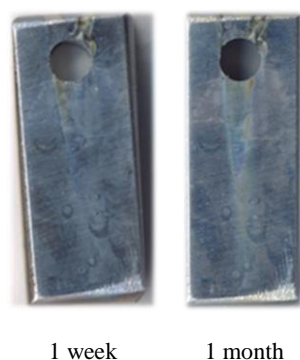
Figure 5: Surface appearance of CRA after one week and 30 days exposure in Cu-containing geothermal water
