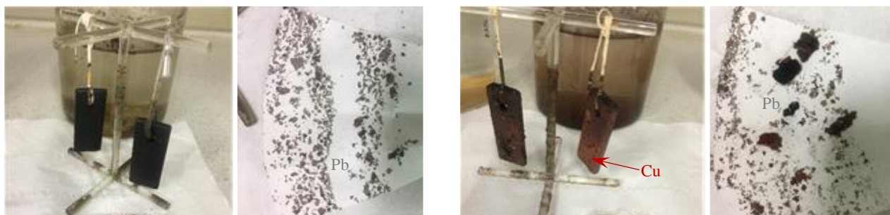
Figure 10: Appearance after 100 d exposure of C-steel in Pb- (left) and Pb/Cu- (right) solution at 150 °C with precipitations filtered from the solution
