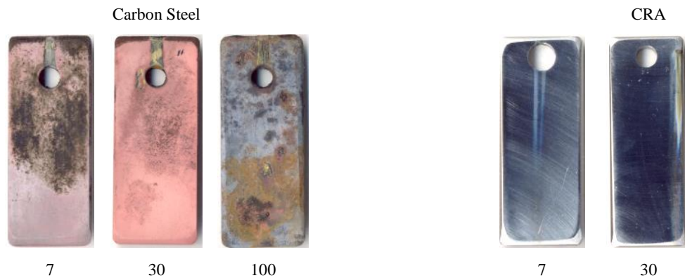
Figure 8: Specimens after 7, 30 and 100 days in Pb/Cu-containing solution at 150 °C
