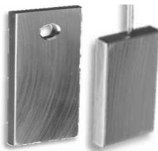
Figure 2: Specimen design for exposure (left) and electrochemical (right) tests
