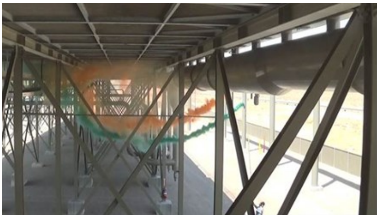
Figure 10: Air inlet streamlines in cross wind WGVS
