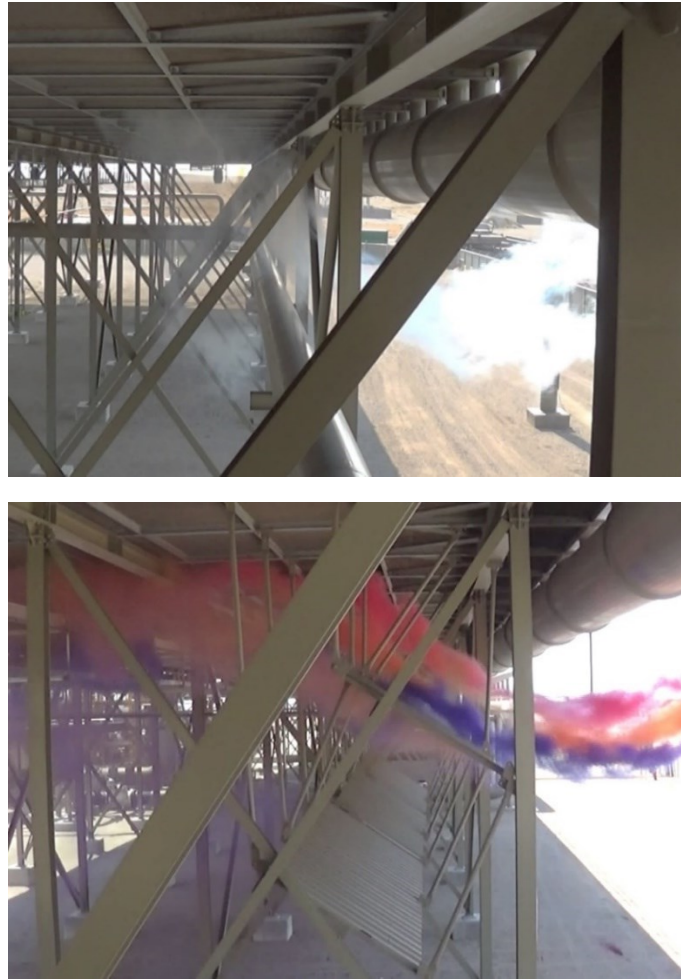
Figure 7: Air inlet streamlines in no wind conditions, WGV bays vs standard bays
