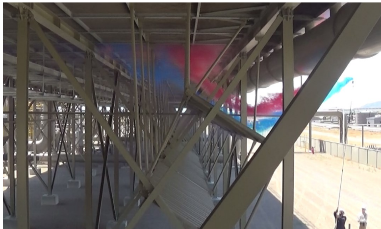
Figure 10: Air inlet streamlines in cross wind WGVS
