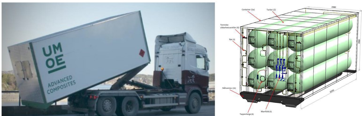
Figure 8: Trucking hydrogen vessel bundles from production site to usage sites is common for hydrogen transportation (UMOE Advanced Composites, 2017), (Suomilammi, 2018)
