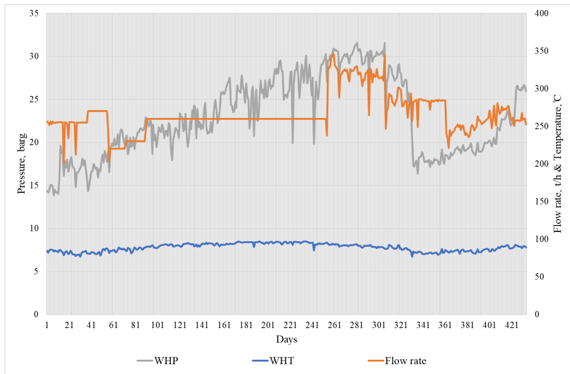
Figure 4. Wellhead monitoring example of one of the reinjection wells for a geothermal power plant.
