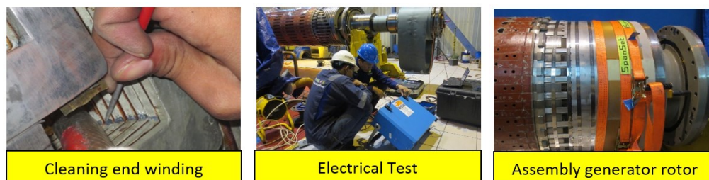
Figure 13: Cleaning hardens the contaminant, electric test and assembly new retaining ring insulation.
