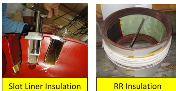
Figure 10: Preparation insulation material (slot liner and retaining ring) before being to do the assembling of slot liner and retaining ring and coil and retaining ring.
