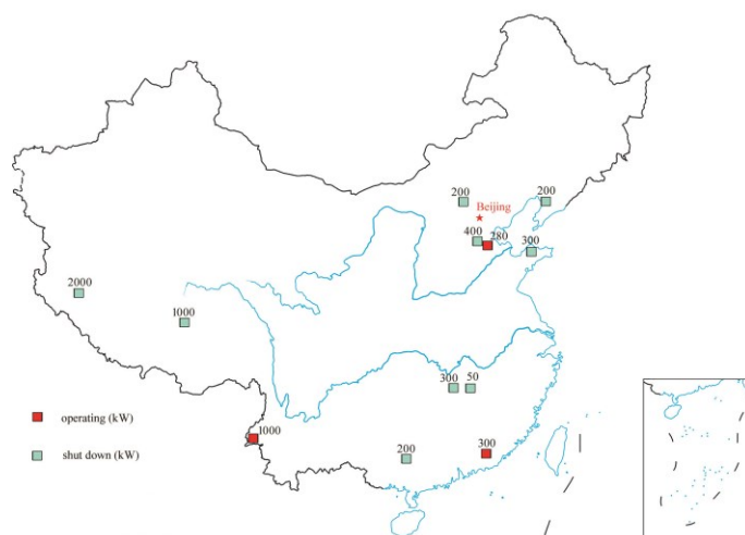
Figure 1: Distribution sketch of medium-low temperature geothermal power plants
