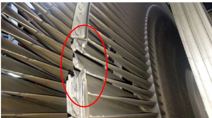
Figure 6: Rubbing at Shroud #4 turbine.
