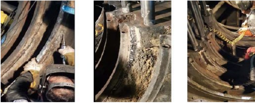
Figure 4: Corrosion product founds at lower casing Turbine.
