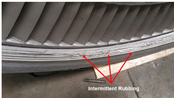
Figure 7: Rubbing at Seal Strip area
