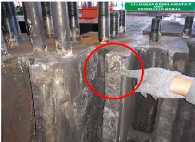
Figure 5: Corrosion at Diaphragm's support plate and Lock Pin. This corrosion makes wear in the diaphragm area.
