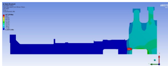
Figure 12: Finite element analysis on stubbed rotor connection. Red color shown the critical area of stubbed material.
