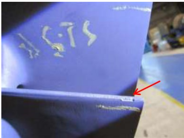
Figure 8: Erosion at Stellite Blade row #5 and #6.
