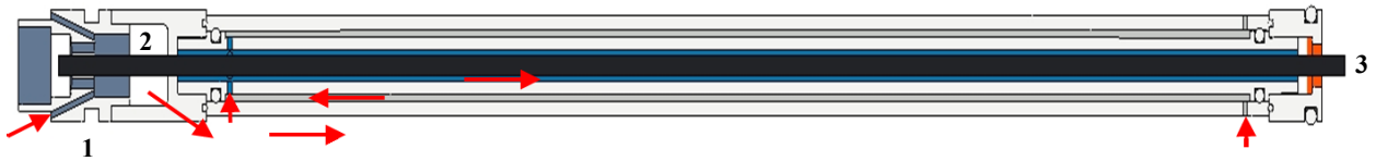
Figure 2: Sectional drawing of additional flow channel which is installed in the PEEK tube (Fig. 1) and which is surrounding the heating rod (3). Arrows mark the flow direction starting from the mixer (1). The position of the thermocouples is indicated by (2).
