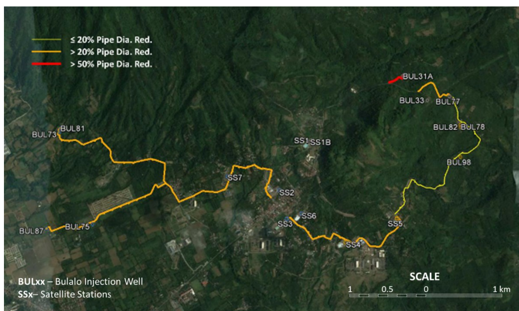
Figure 15: HBIS network sections with scale build-up, color coded based on percentage of pipe diameter occupied by scale.
