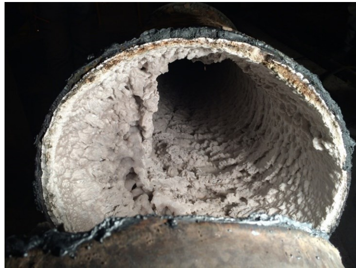
Figure 14: Scale blockage observed within the WS-06 steam line in 2015.
