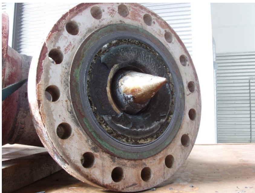
Figure 3: This picture shows how a spiral-wound steel gasket seals both the flange and the orifice plate.
