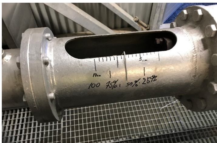
Figure 4: The coupling tube with improvised position indicator.
