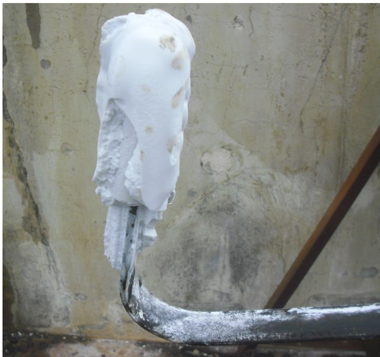
Figure 9: Soft silica scale below brine level in barometric pipe.
