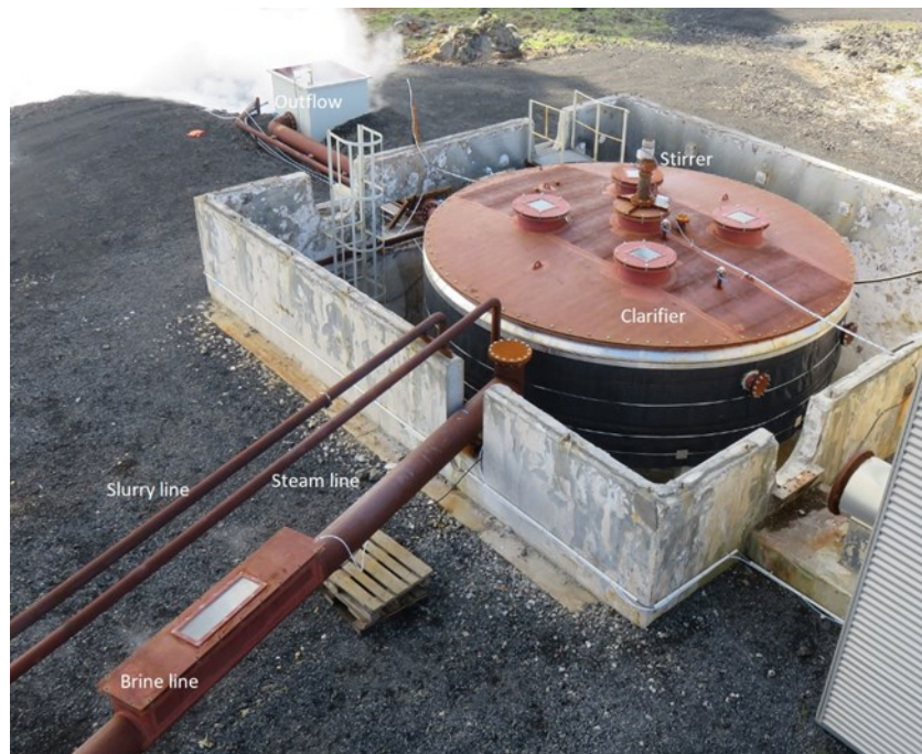
Figure 6: Clarifier and brine, slurry and steam lines from the reactor.
