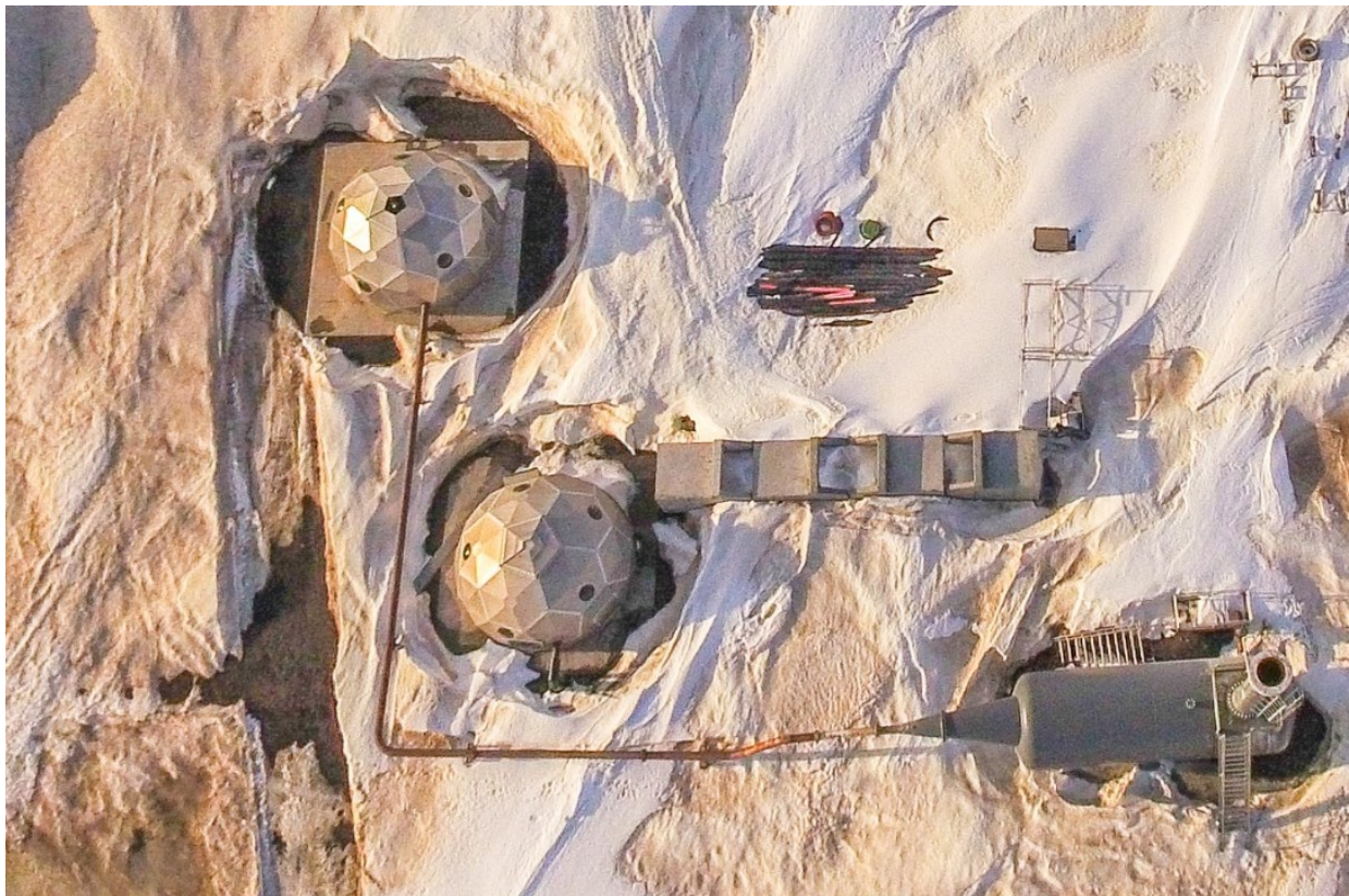
Figure 4: Aerial view of the apparatus in Beistareykir, Iceland. The flowline follows the piping from hole ÞG-18 to the steam separator.
