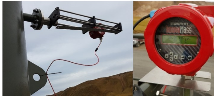
Figure 6: Vortex meter used in the experiment. Picture to the left shows how the Vortex meter is connected to the steam separator.
