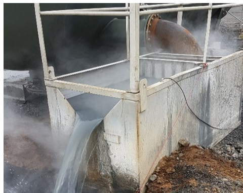
Figure 7: The water weir used in the experiment. The separator water from the separator flows into the weir.
