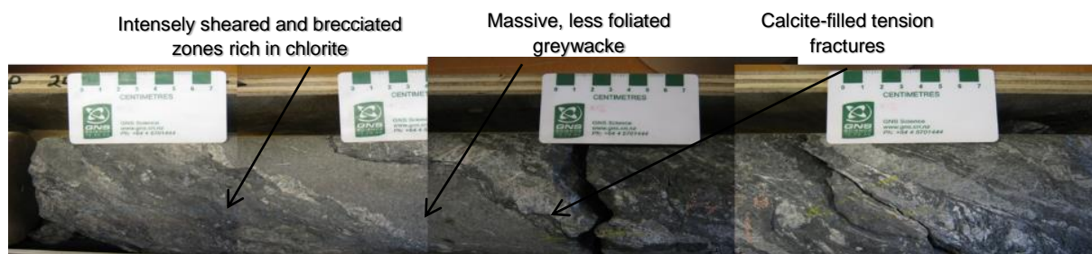
Figure 3: Core sample retrieved from \sim 2500 m in the greywacke, the main injection formation.
