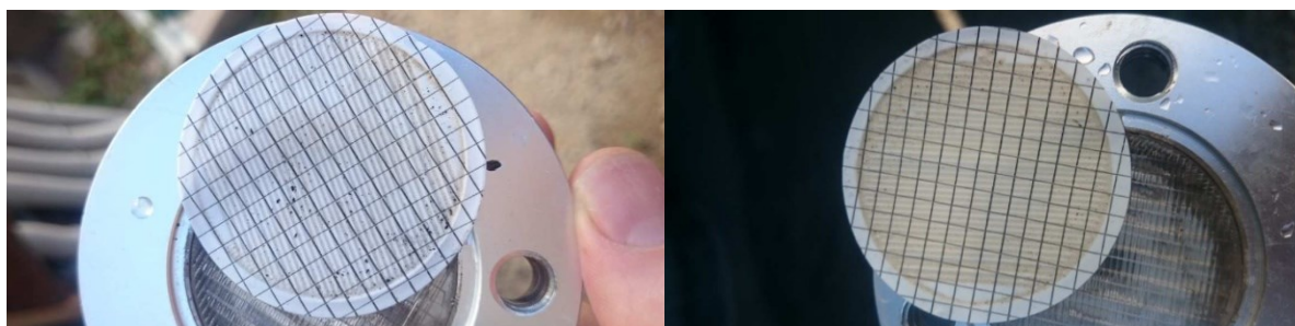
Figure 4: MFI testing on 0.45 micron paper of groundwater at production borehead (left) and post filter (right)
