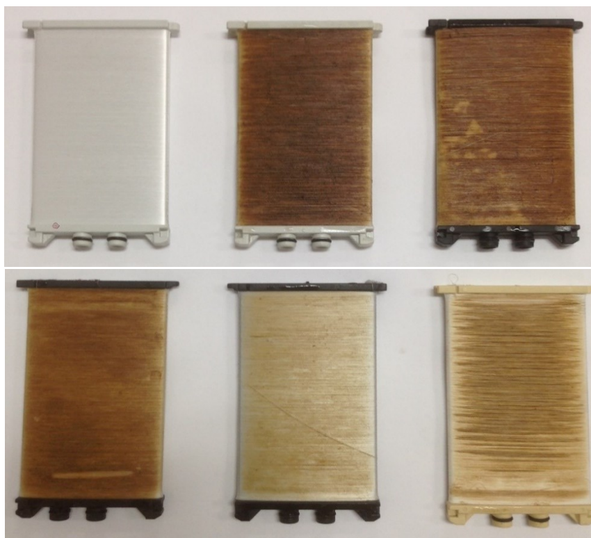
Figure 9: Testing undertaken by the filter contractor (Amiad Water Systems) using microfiber filter cassettes confirmed a minimum of 5-micron filtration and optimal of 1-micron filtration was desired (from top left to bottom right, New, 20-micron, 10-micron, 7-micron, 3-micron and 2-micron)
