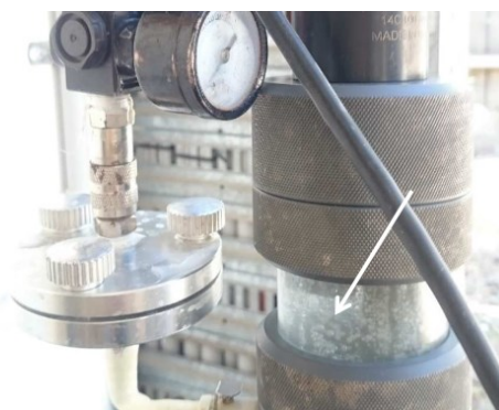
Figure 5: Dissolved Gas in groundwater degassing in flow-through sampling cell at low supply pressures (<1 bar)
