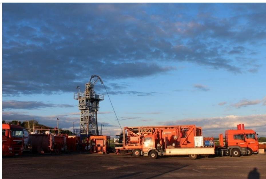
Figure 2: Soft stimulation operations at Rittershoffen geothermal site in the Upper Rhine Graben where injectivity was improved by a factor 4 (Baujard et al., 2017).
