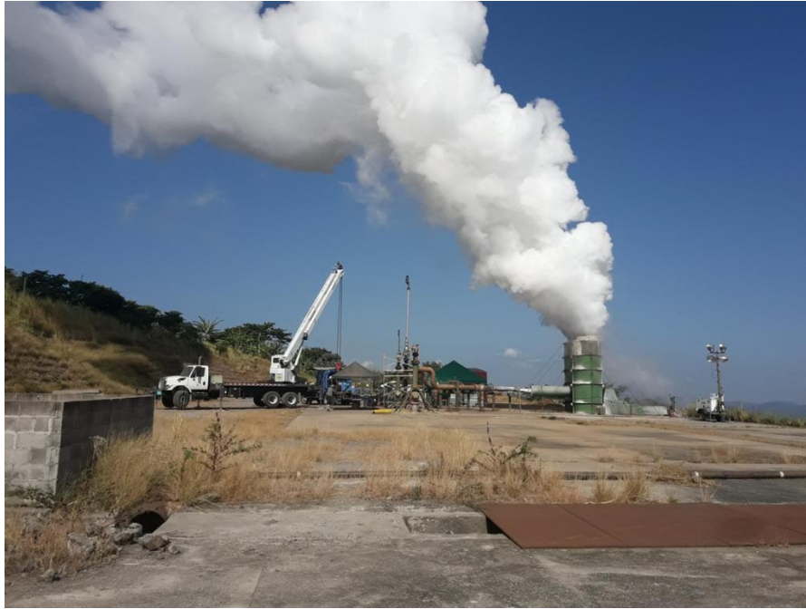
Figure 3: Discharge test facilities in a geothermal well
