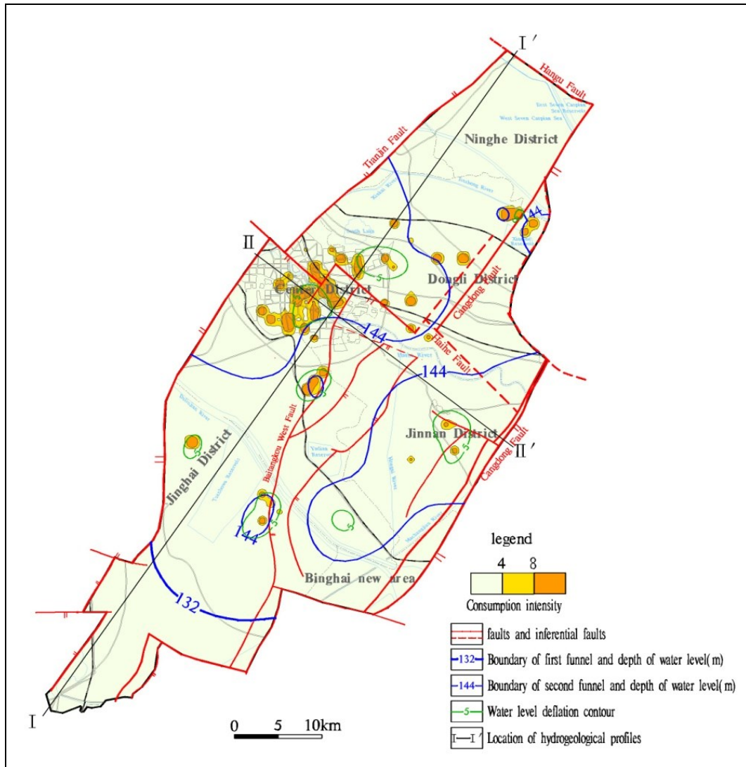
Fig. 4 the consumption intensity of Wumishan group corresponds to the water level descending funnel in 2018
