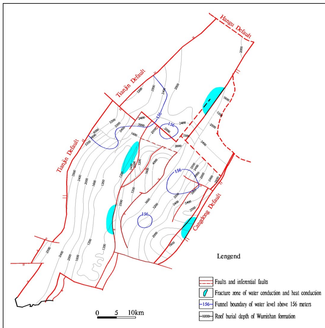
Fig. 9 Corresponding relations among the roof buried depth of Wumishan group reservoir, fracture and the water level falling funnel
