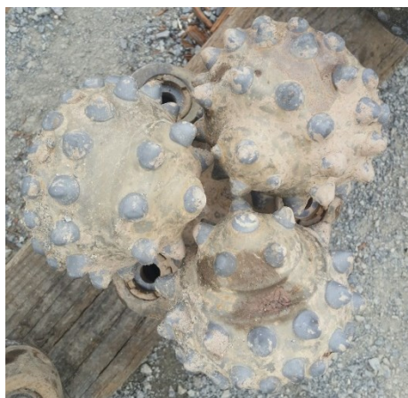
Figure 4: Pulled bit, showing excessive wear, including broken teeth and dull gauge.
