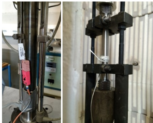
Figure 4: Actual temperature measurement of the sample during the experiment with type E thermocouple.
