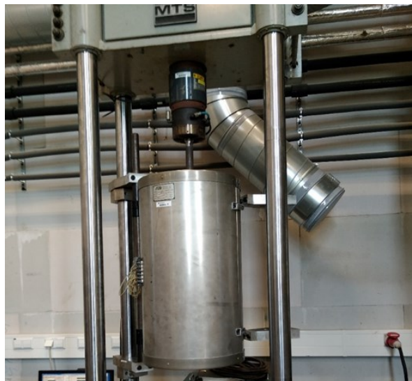
Figure 1: MTS tensile rig with integrated oven.
