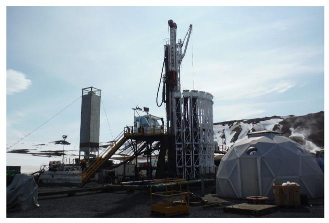
Figure 5: Rig Sleipnir on the first well, THR-11, next to existing well (wellhead inside the igloo). May 2016.
