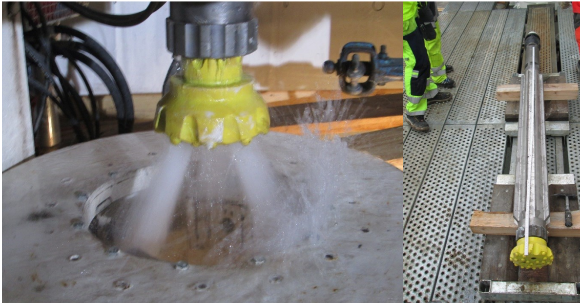
Figure 3: left: water hammer drill bit (203 mm diameter) in action, right: drill bit, hammer case with steering ribs and check valve.
