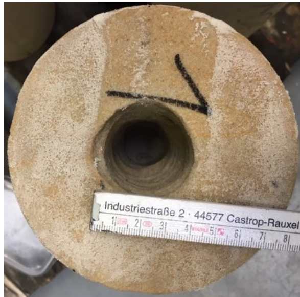
Figure 2: Photo of Gildehaus specimen after experiment with rotating nozzle design.
