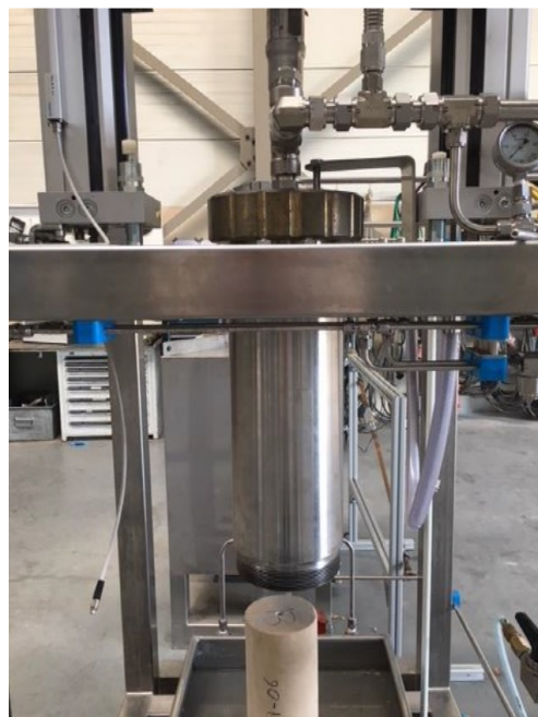
Figure 1: ‘iBOGS mini’ autoclave being used for jetting experiments under reservoir type conditions.
