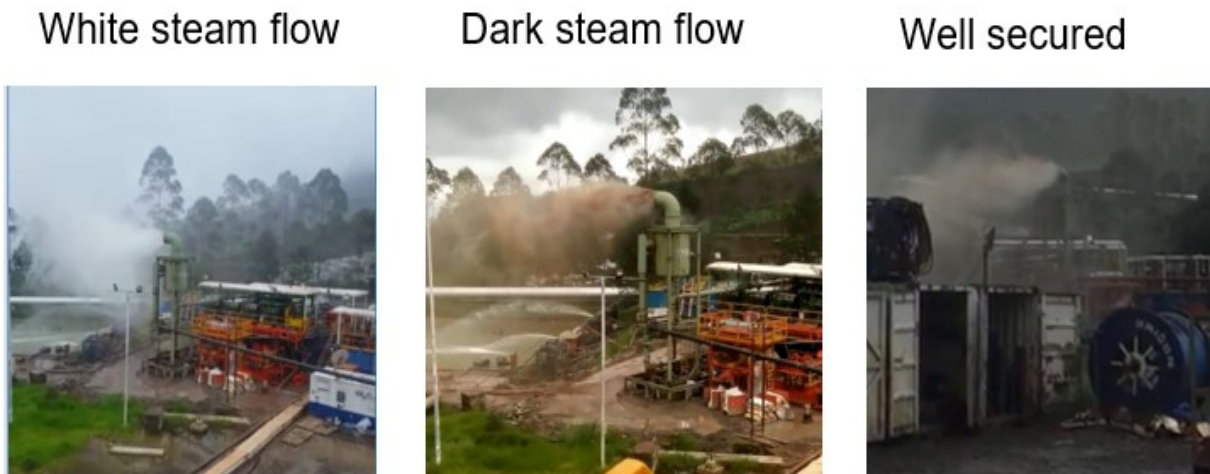
Figure 7: MBD-8 initial white steam started flowing from separator and changed to dark brown steam.
