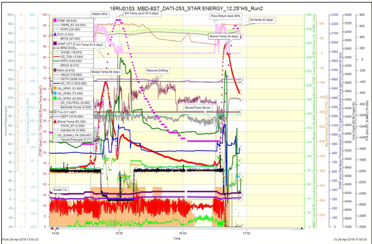
Figure 6: Two well control events in MBD-8 parameter plot from initial of steam flow condition until well secured
