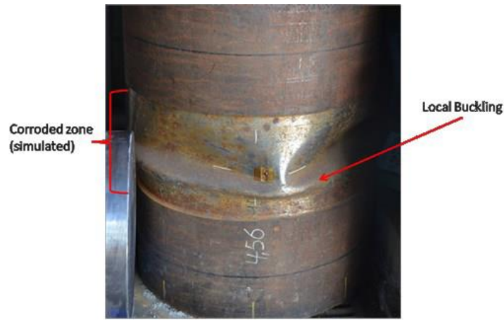
Figure 6. Example of local inelastic buckling (after Teodoriu, 2015)
