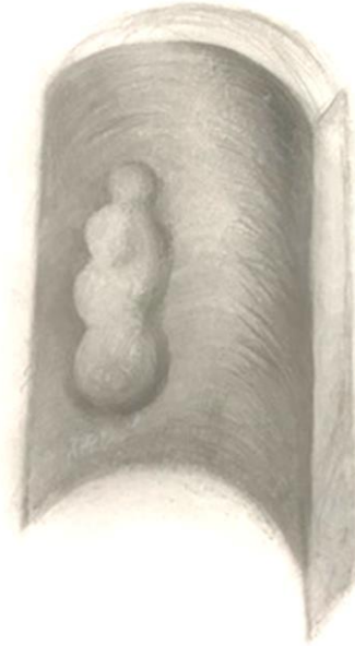
Figure 8. Illustration of APB induced collapse. Note the inward protrusion at the location of the collapse. There is no failure, but the protrusion compromises drift.
