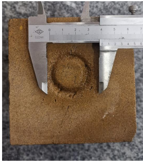
Fig. 10 SAWJ rock breaking effect
