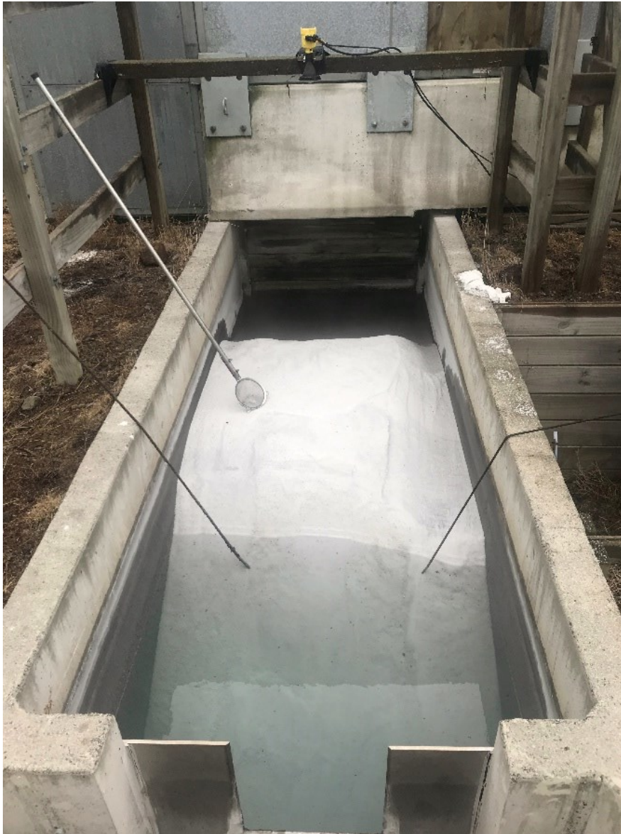
Figure 2: Over 5m 3 scale removed from WK267 with the CTH, deposited in the weir box beyond the silencer.
