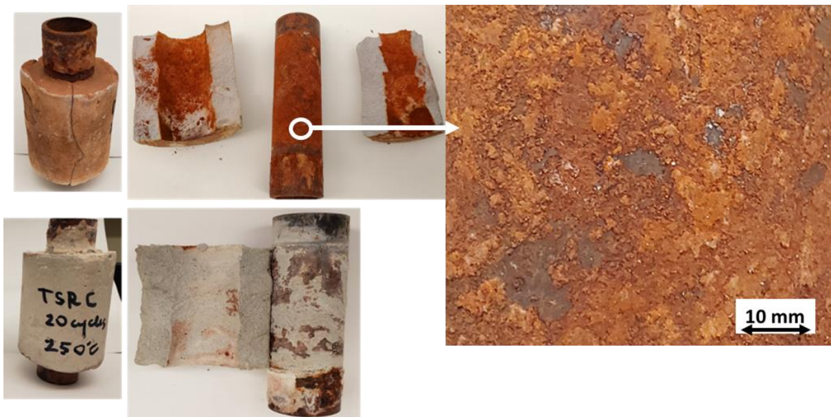
Figure 9: Appearance of OPC/SiO 2 sheath samples (top) and TSRC sheath samples (bottom) after 20 severe TS cycles.
