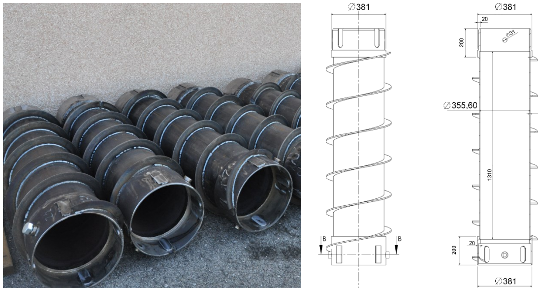
Figure 5: a) Manufactured enlarged easy drill segments (left) b) Technical drawing of the hollow auger drilling tools (right). Both figures (Bernini, 2016))
