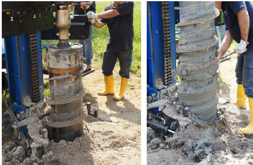
Figure 7: Enlarged Easy Technique during the drilling at the Molinella (Italy) test site. a) Drilling in more sandy units (left). b) Decoupling of two ‘Enlarge Easy Drill’ segments after penetrating more plastic units.
