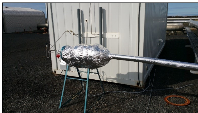
Figure 6: Autoclave systems for material testing. On the left the high temperature autoclaves and on the right the autoclave used for well head condition testing.
