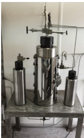
Figure 6: Autoclave systems for material testing. On the left the high temperature autoclaves and on the right the autoclave used for well head condition testing.
