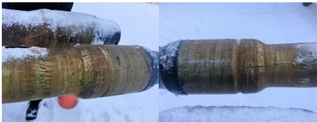
Figure 7. Damaged drill pipes after having been stuck in a keyhole for 3 days
