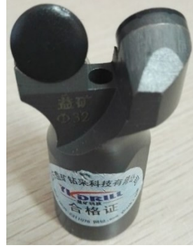
Figure 2: Micro-PDC bit used in the experiment.
