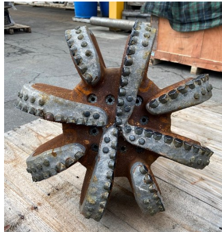
Figure 6: 20¾ in. TKC89 drill bit showing good condition with minor chipping on the gauge. The below performance charts and results were compared on packed rotary assemblies and drill off tests were performed to optimise performance depending on hole conditions.
