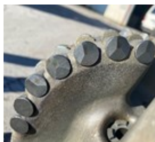
Figure 12: 12¼ in. A2 run on TH28 was pulled with no cutter wear after drilling 366m through Ignimbrite.
