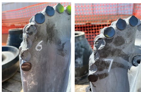
Figure 5: 12¼ in. A1 design drilled 1351m through hard volcanic rocks at 19m/hr. Considerable impact damage can be seen on the shoulder and gauge region.
