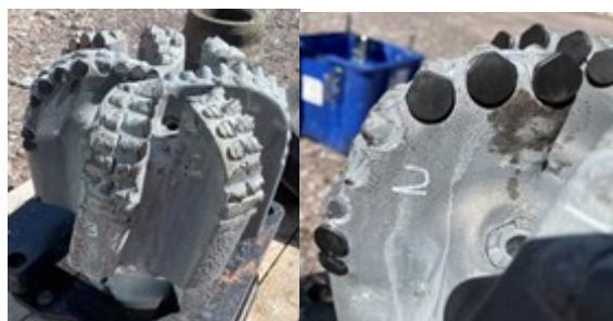
Figure 11: 12¼ in. FTKC76 A1 drilled on TH24 was pulled with a ring out on the shoulder after drilling 1351m through Ignimbrite.
