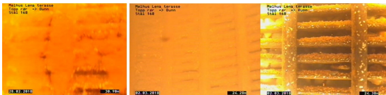
Figure 4: Picture at left: The well screen is tight before rehabilitation in February 2018 when the water was flowing over. The blurry picture is caused by a thin film on the camera lens. Picture in the middle and at the right: Video inspection of the well screen after jet flushing with mixed results. The pictures are within 10 centimeters, and large parts of the screen is still clogged with precipitated iron oxides (middle), while the natural filter of sand and gravel can be seen in some parts (right picture)
