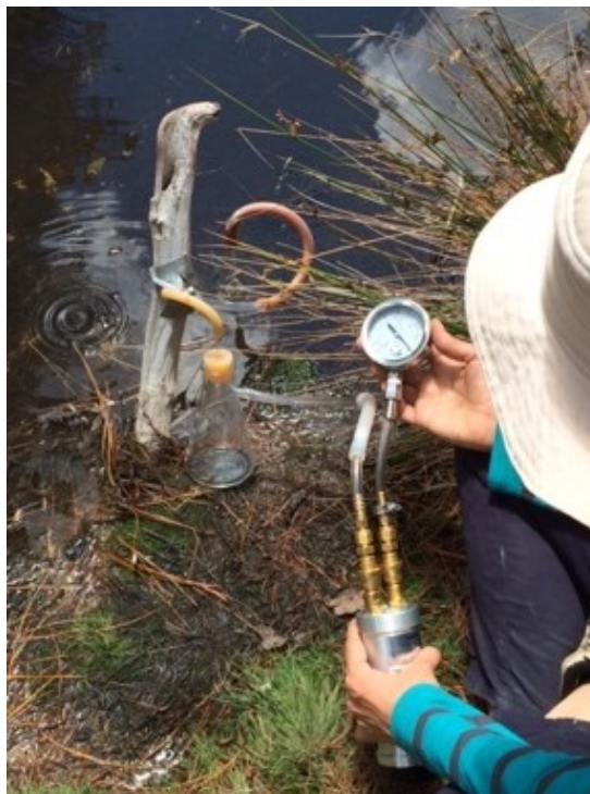
Figure 4: Gas sampling collection system used for the radon monitoring by using the Lucas tube 600A.
