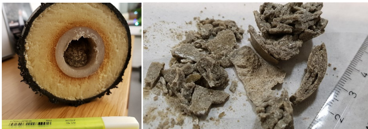
Figure 2. The calcite scales collected from the surface pipes within Selfoss district heating system several kilometers from the pumping station.
