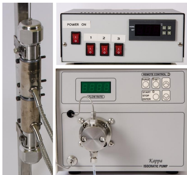
Figure 1: Flow-through EHPV (left) and temperature control panel (upper right) of the HPLC pump (lower right) used in laboratory experiments
