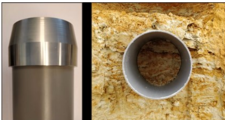
Figure 3: Sampling tube for undisturbed samples (left), allowing to gather samples of unconsolidated sands whilst keeping sedimentary structures intact (right).
