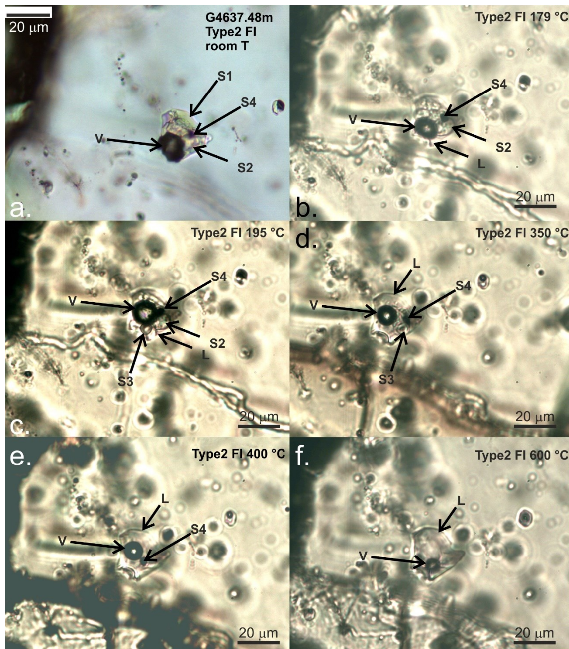
Figure 4: Phase transformations in Type2 fluid inclusions during heating experiments. Photomicrographs were taken in plane polarized light at a) room temperature, b) 179 °C (S1 already dissolved), c) 195 °C, d) 350 °C (S2 already dissolved), e) 400 °C (S3 already dissolved), f) 600 °C (S4 already dissolved). Note the change of the shape of vapor bubble between room temperature and 179 °C.
