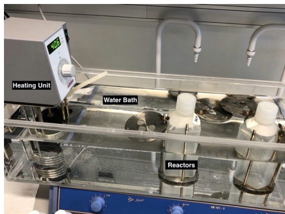
Figure 3: Setup used for silica scaling experiments.
