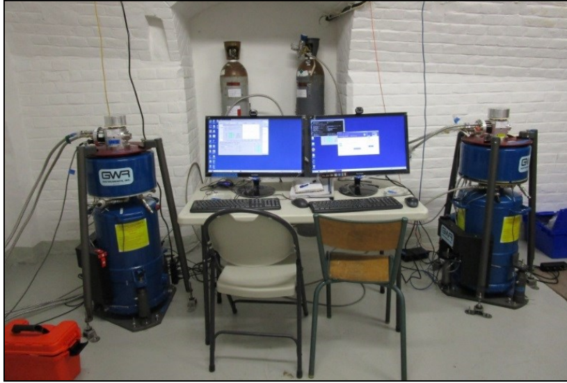
Figure 1: Measuring setup for iGrav032 and iGrav015 at the underground observatory J9 near Strasbourg, France.
