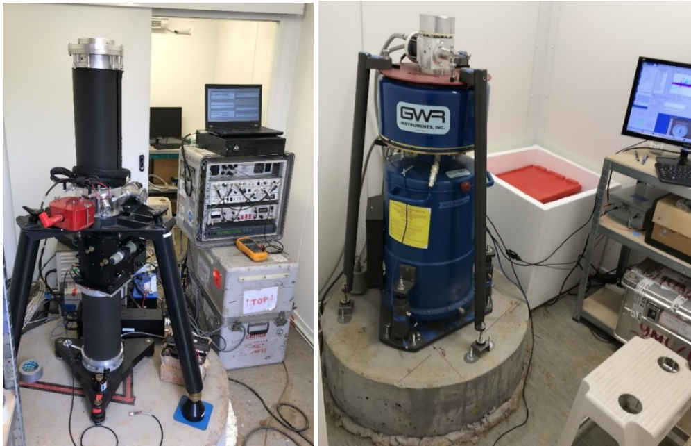
Figure 3: Typical setup of a FG5 absolute gravity meter (left) and an iGrav SG on the pillars in the container. The compressor for the iGrav is placed in the front compartment to minimize vibrational noise from its operation. On each relative gravity meter pillar, there is also a broadband seismometer placed. (pictures: K. Erbaş)
